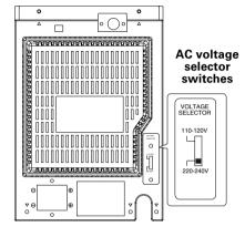
Move switch lever to match your line voltage with a small screwdriver or other pointed tool.
